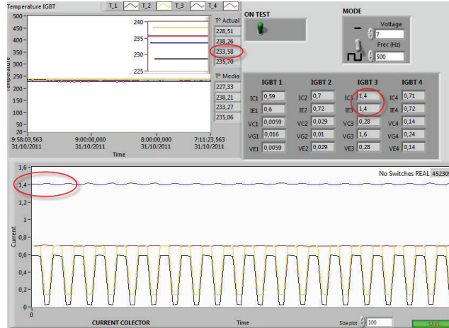
FIGURE 8: Short circuit fault current in IGBT 22.
