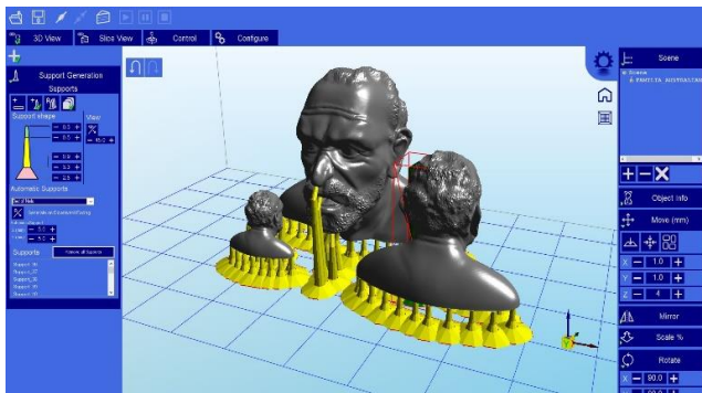
Figure 3: Preparation in the Creation Workshop program of the 4 models in different sizes for printing in resin using the WANHAO Duplicator 7 printer.
