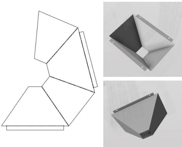
**Fig. 6** Development drawing of the reflection cover
