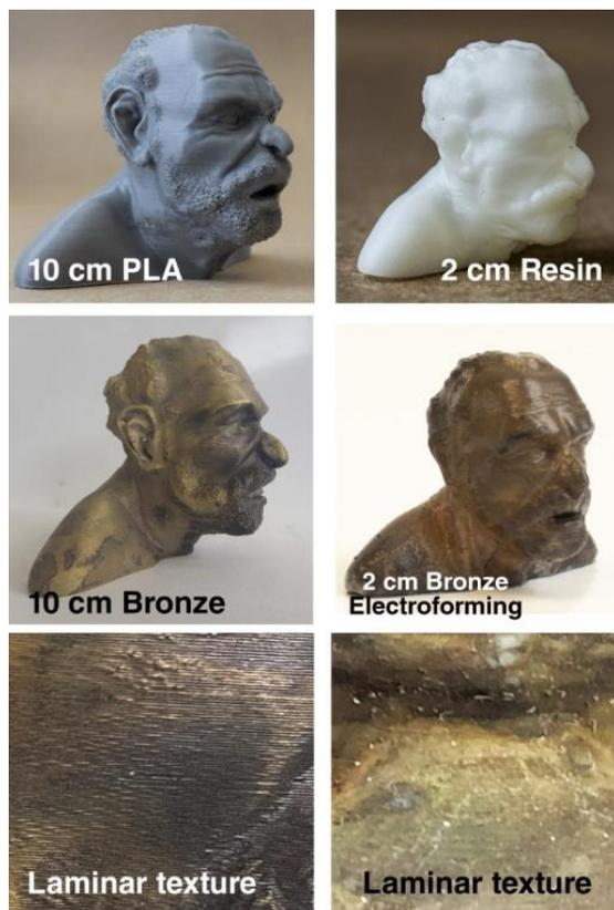
Fig 1 Examples of figures made by PLA and resin molds.
